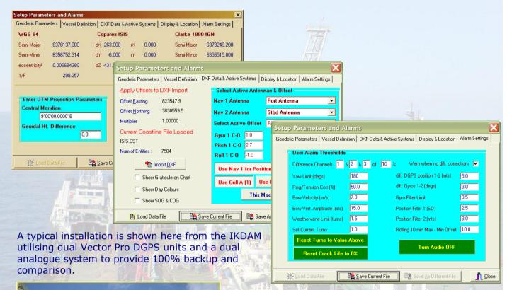
The alarm panel is shown here, the items in red are outside of limits and the cross to the right of a non-red item indicates that it was outside limits but has returned inside limits now.
